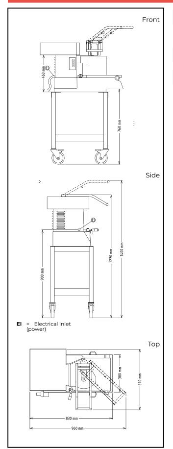
Electric Supply voltage: 380-415 V/3 ph/50 Hz Electrical power, max: 2 kW **Total Watts:** 2 kW Capacity: Performance (up to): 700 kg/hour Key Information: External dimensions, Width: 610 mm External dimensions, 830 mm Depth: External dimensions, Height: 1400 mm
